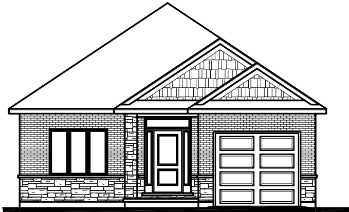
FRONT ELEVATION- UPGRADED BRICK OPT.
